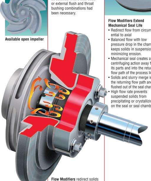
and slurry away from seal and
