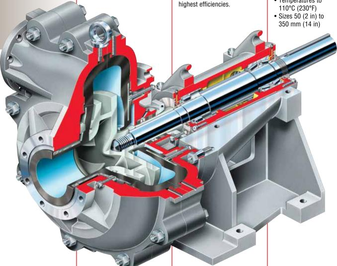
Dual Casing provides access to elastomeric or hard metal liners for inspection or replacement. Machined mating faces provide proper liner compression. Both the radial joint and piping connections are complete through-bolt designs for ease of disassembly.
