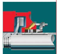
Optional Expeller Seal uses centrifugal force to expel fluid from the seal chamber. Recommended for applications in which abrasive particles cause frequent packing failures, clean water is limited, or product dilution is not tolerable.
